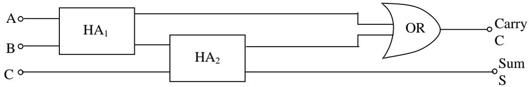
**Fig 2 (b): Full – adder Logic Symbol**
