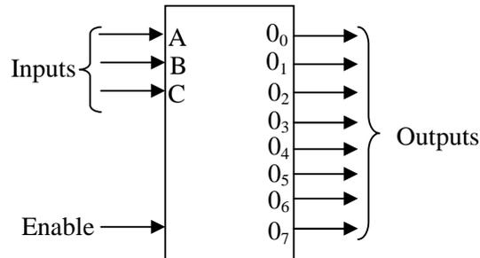
**Fig c Block diagram of 3 to 8 bit decoder**
