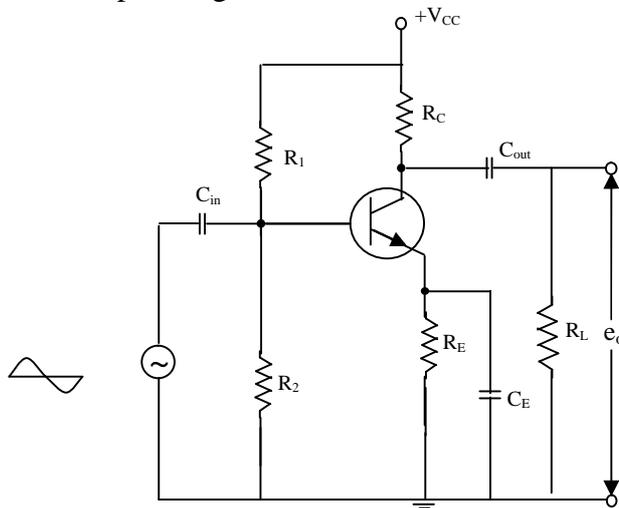
**Fig 1 A single stage R-C coupled amplifier.**
