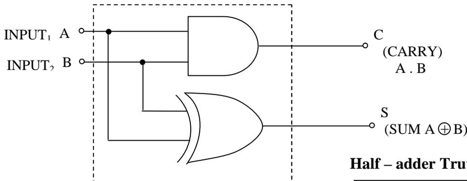
**Fig 1(a) Half-Adder Logic circuit**
