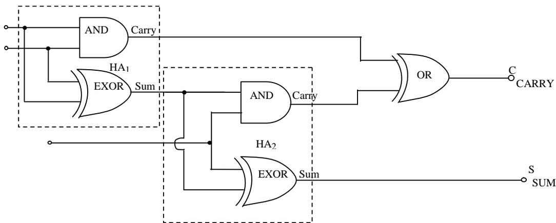
**Fig 2(a) : Full – adder Logic diagram**
