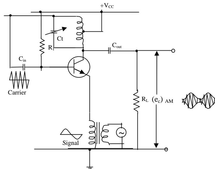
**Fig 1.3 An amplitude-modulated oscillator****Observations :**
